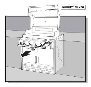
11. Lift and twist the burner assembly slightly, to separate the Crossover® tube (a) from the burners (b).
